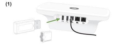
Remove cap and insert USB Adapter
