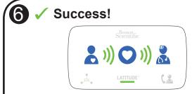
If your lights are lit as shown above, setup is complete! The lights will turn off automatically after 2 minutes.
