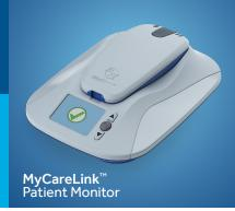
When an error condition occurs with the MyCareLink $^{\text{\tiny M}}$  patient monitor, the display screen provides a four digit code, along with an animated graphic to help patients resolve the error. These error codes indicate action that needs to be taken with the monitor; the error codes **do not** refer to the patient's implanted heart device.
